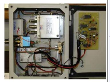
transverter and the power amplifier in a weather proof box but also included all the switching and a sequencer to add further protection to the package. This arrangement also enabled Paul to much less expensive LMR coax rather than wave guide to all that 10GUz energy to the antenna and back down to tower To his IF radio.
